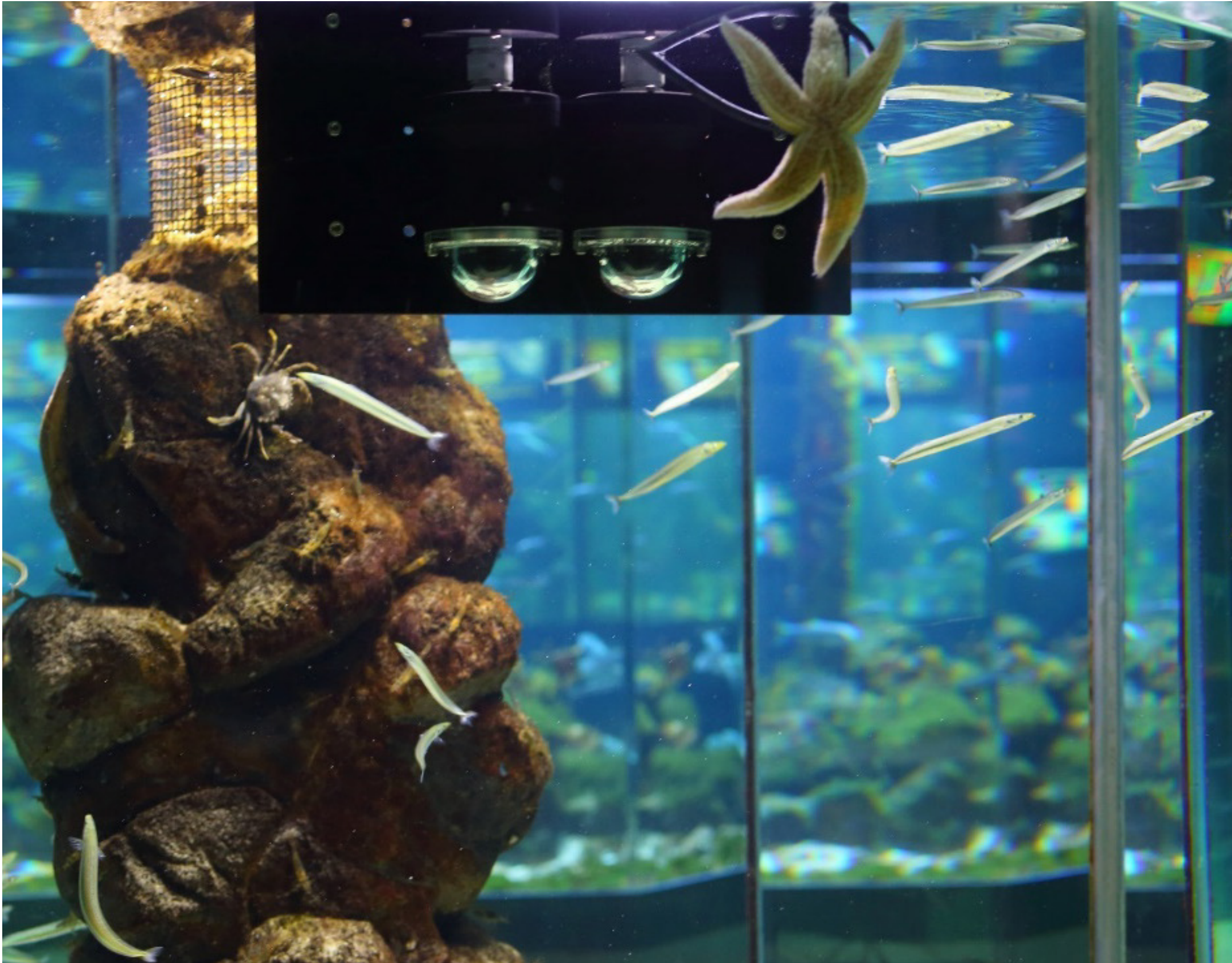
Figure 2. FishGuard stereo camera setup with 2 parallel cameras.
